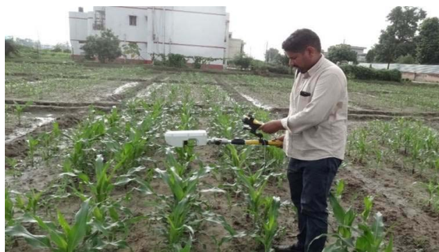
Photo 58. NDVI reading being taken using Green Seeker
