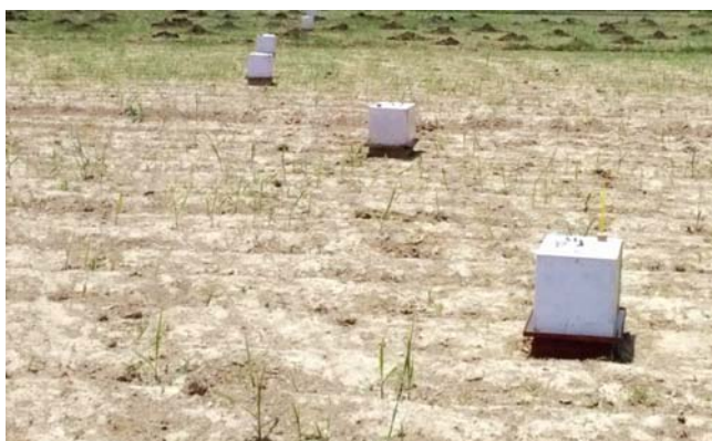
Photo 21. Measurement of GHG emission in sugarcane crop
