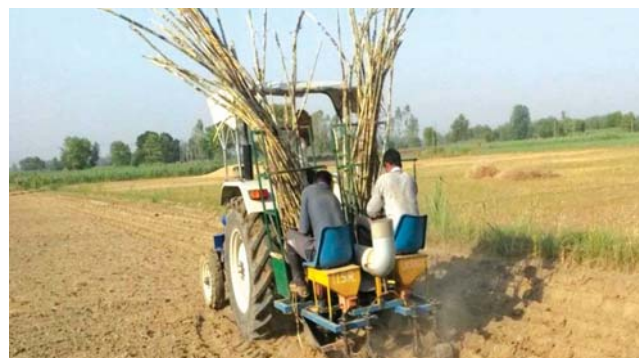
Photo 19. Demonstration cum evaluation of sugarcane cutting and planting device
