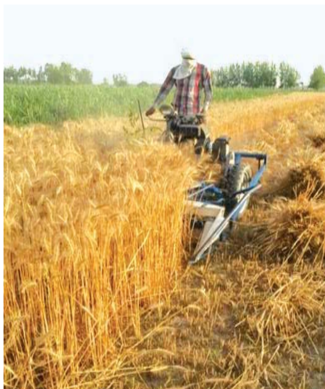
Photo 18. Demonstration cum evaluation of reaper binder for harvesting of field crops
